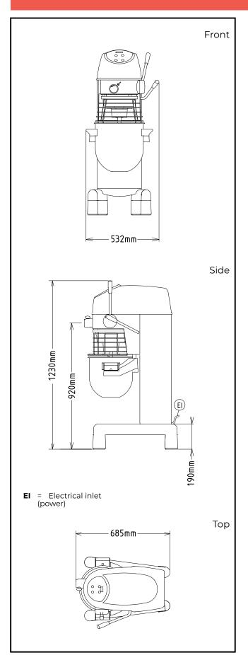
Electric Supply voltage: 220-240 V/1N ph/50 Hz Electrical power, max: 0.75 kW 0.75 kW **Total Watts:** Capacity: Performance (up to): 6 kg/Cycle Capacity: 20 litres Key Information: External dimensions, Width: 521 mm External dimensions,
